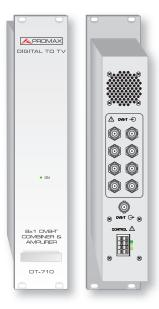
The **DT-710** is a combiner with 8 inputs and an output designed to mix output RF signals of **COFDM** modulators and transmodulators with DTT channels available in the area. The system provides an amplified output of 114 dB $\mu$ V (+6 dBm) frequently required in **SMATV** systems.
